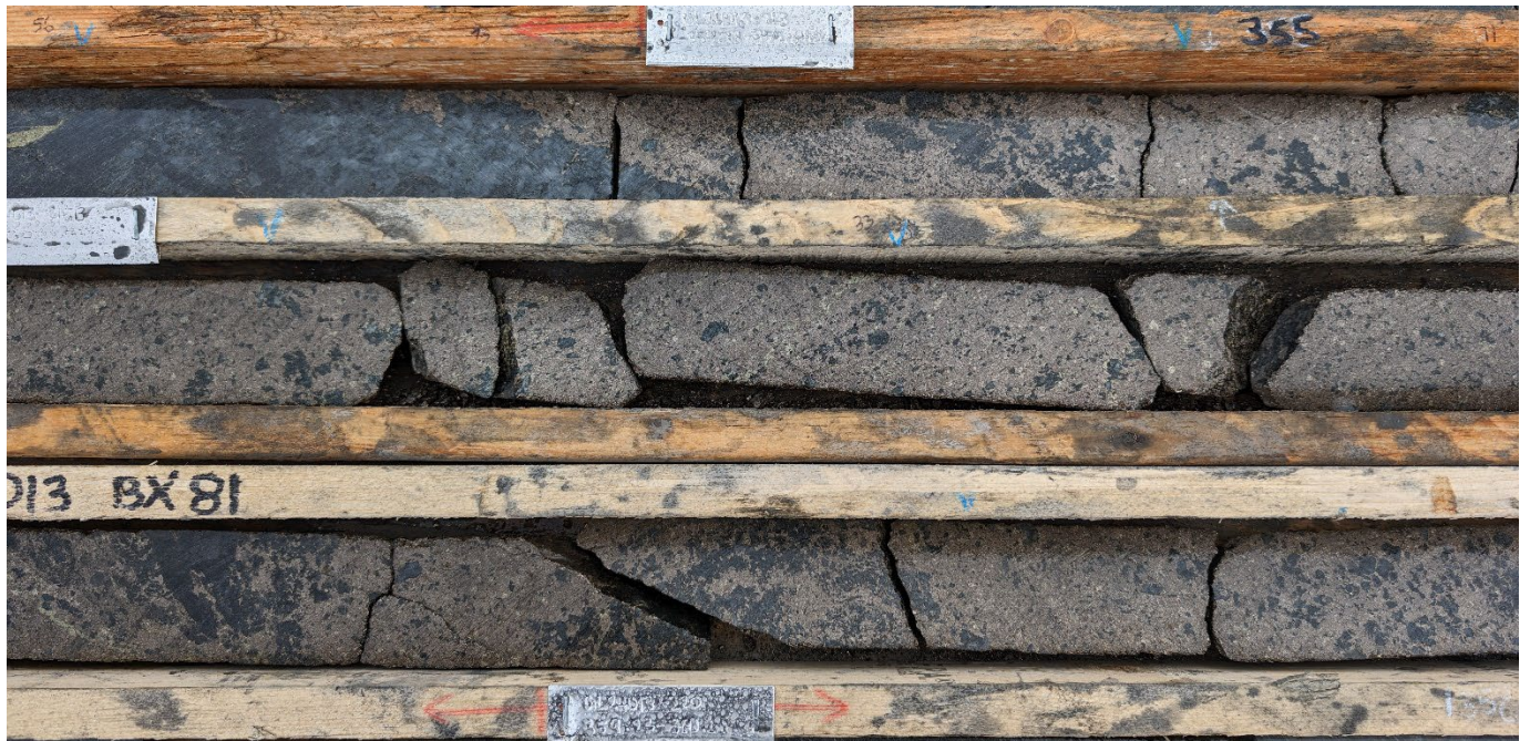
Photo – 3: Detailed Photo Semi-Massive to Massive Sulphide Mineralization (cut core); drillhole GL24013 starting @ 354.75 meters
