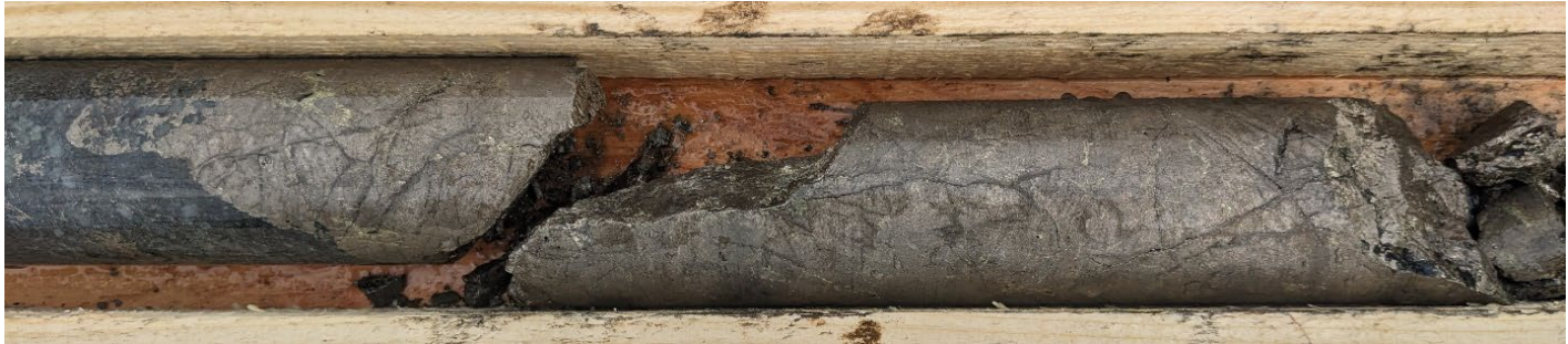
Photo 5 Disseminated, Coarse Pentlandite Drillhole GL23003 at drillhole depth ~ 143 meters
