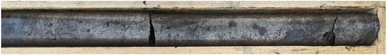
Photo – 4: Drillhole GL23008 Massive Sulphide Vein with Interpreted Loop Pentlandite, Chalcopyrite Texture at drillhole depth ~255 meters
