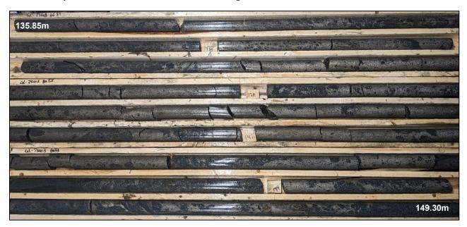
Photo – 2: Massive Sulphide Mineralization; drillhole GL23003 at 130.45m, pentlandite, chalcopyrite noted in drillhole log; interval 130.40 – 130.95m assayed: 2.38% Ni, 0.38% Cu, 0.19% Co, 0.26 g/t 3PE / 0.55m
