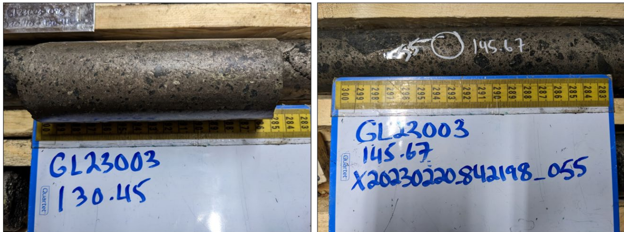
Photo – 2: Detailed Massive Sulphide Mineralization (left, 130.45m) Brecciated, Massive Sulphide Mineralization (right, 145.67m) Drillhole GL23003
