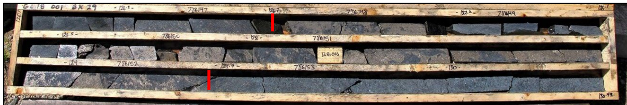
Drillhole GL18-001; semi-massive to massive Ni-Cu+Co sulphide mineralization at 126.7 – 129.4m
