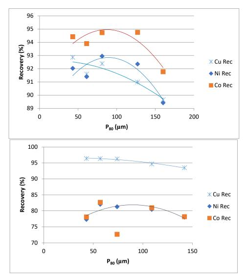
Figure 13-3 Grind-Recovery for Grab Sample (Top) and Drill Core Sample (Bottom) Composites
