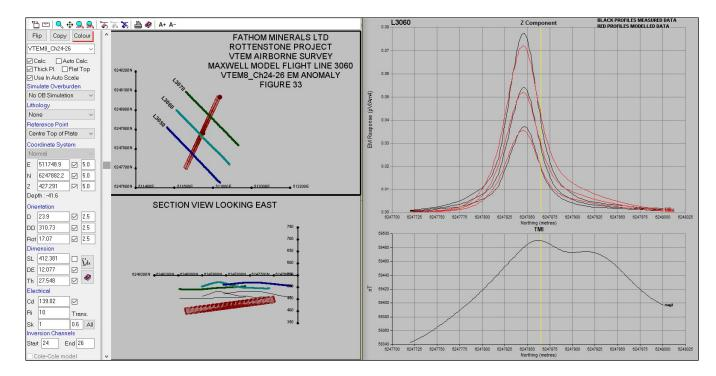
Figure 10-11 VTEM-8 Conductor Maxwell Plate Model Flight-line 3060
