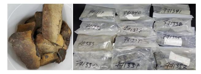
Figure 13-2 Sample material as received: Surface grab sample (left) and drill core (right)
