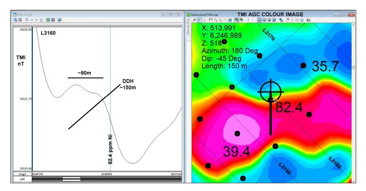
Figure 10-10 NeedAName Coincident Ni-in soil MAG Feature (Mag profile on left, looking north – south; Ni-in soil contour on right)
