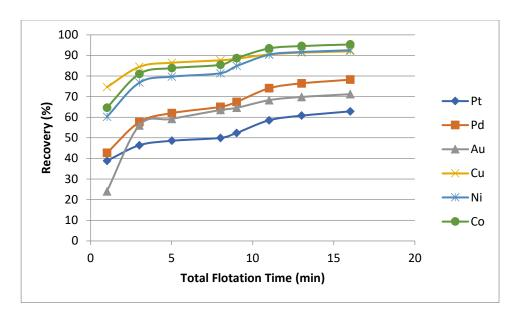
Figure 13-6 Test F1: Grab Sample Flotation Kinetics
