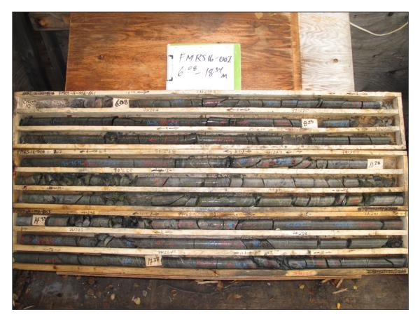
Figure 10-3 Photograph Drillhole FMRS16-002; from 6.08-18.34m (wet)
