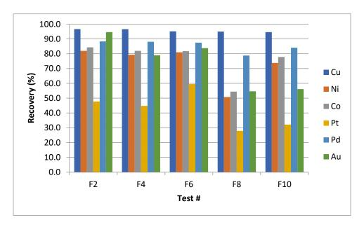
Figure 13-9 Drill Core Composite – Reagent Testing Recovery Response by Metal
