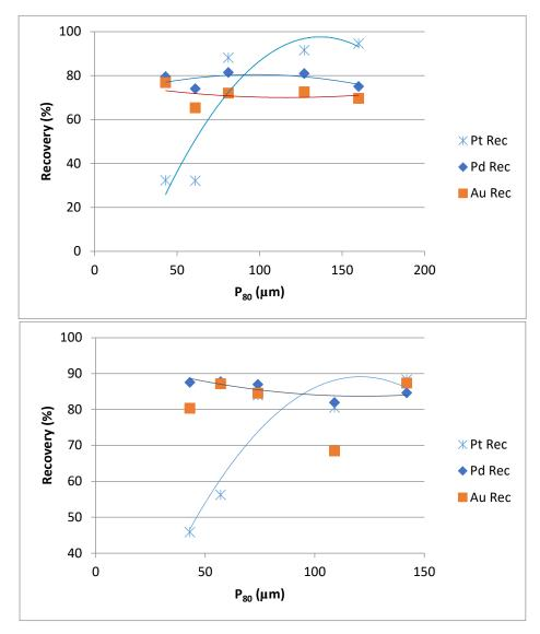
Figure 13-4 Precious Metal Grind-Recovery Curves: Top - Grab Composite; Bottom - Drill Core Composite
