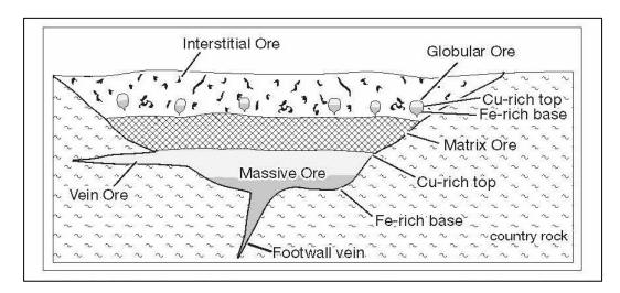
Figure 8-2 Relationship between Massive, Matrix, Disseminated and Vein Sulphides Ni-Cu + PGE Sulphide Deposits; Barnes and Lightfoot (2005)
