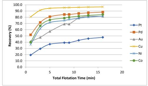
Figure 13-7 Test F2: Drill Core Sample Flotation Kinetics
