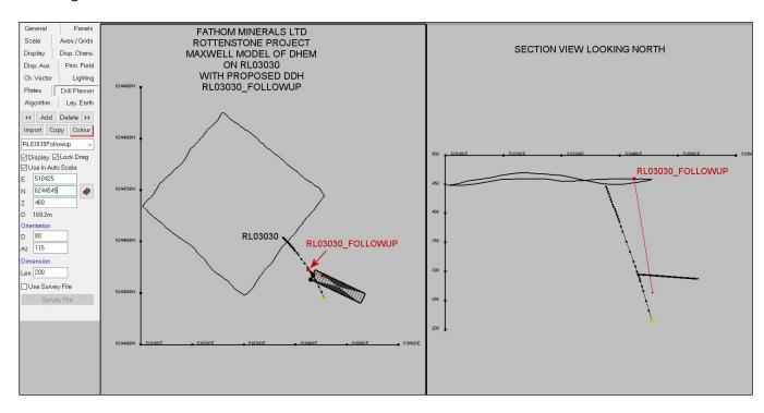
Figure 10-6 Position of BHEM Off-hole Conductor in Drillhole RL03030
