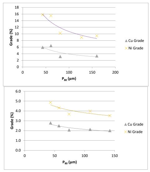
Figure 13-5 Cu-Ni Rougher Grade by Grind Size: Top – Grab Composite; Bottom – Drill Core Composite
