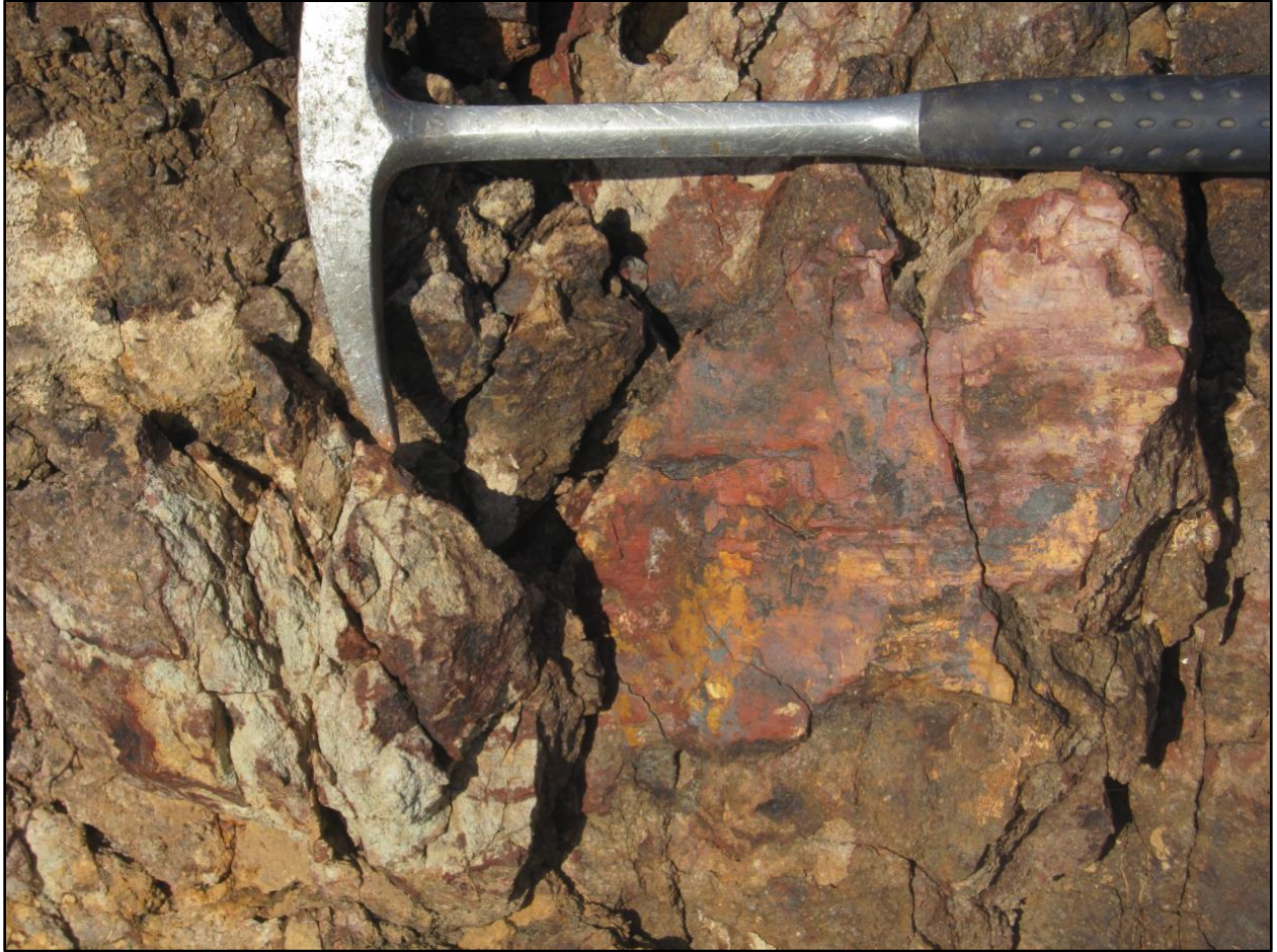
Figure 7-8 Hematitic siltstone with horizontal slickensides.
