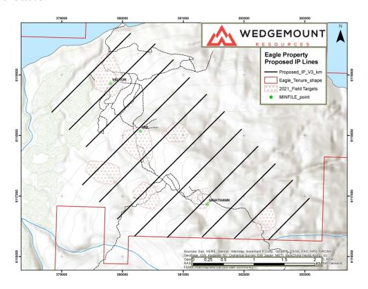
Figure 1: Planned Induced Polarization (IP) survey coverage over priority areas.
