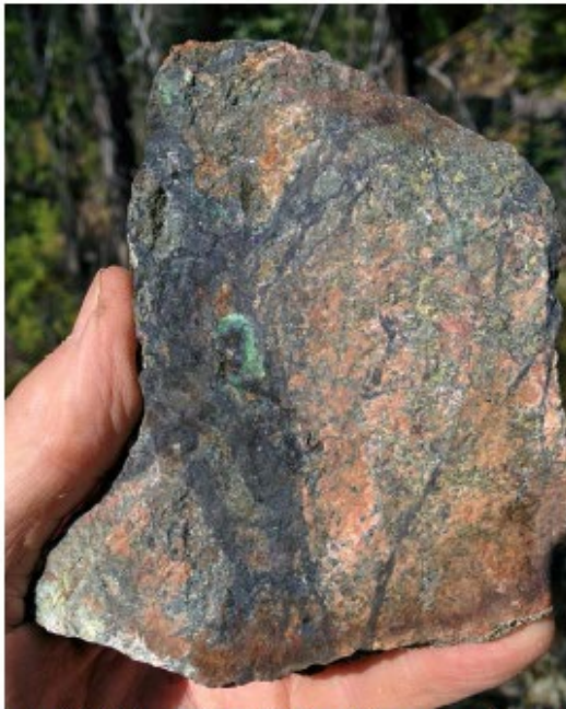
Pervasive K-feldspar(-epidote) cut by magnetite-chalcopyrite veins.
