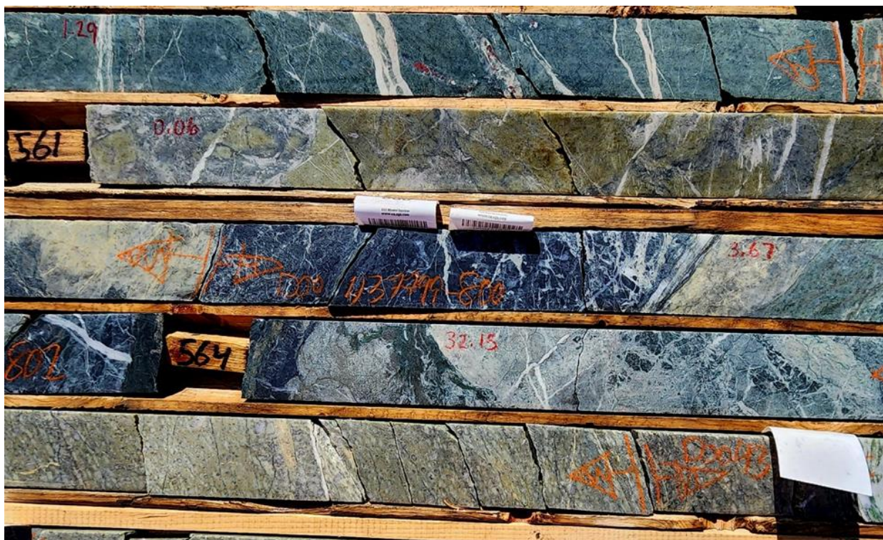
Image 4: Representation of mineralized and altered core from DQ23-05 (10.8 m of 15.8 g/t Au (includes 3.4 m of 27.24 g/t Au)). Highly altered breccia zone containing quartz veinlets, sericite, and ankerite; initial metallurgical recovery of 94%.
