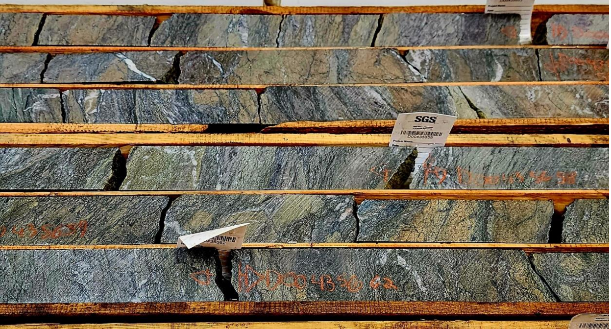
Image 2: Representation of mineralized and altered core from DQ23-02 (10.65 m of 3.97g/t Au (includes 5.0 m of 5.34 g/t Au)); initial metallurgical recovery of 90%.
