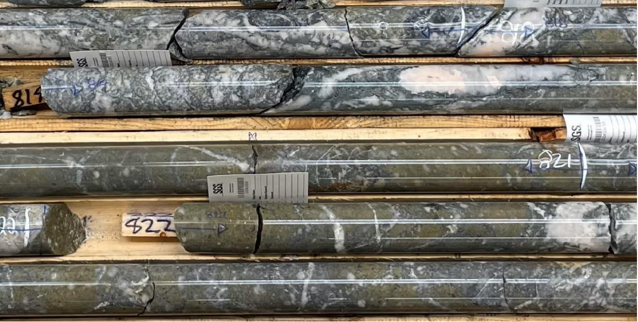
Image 3: Representation of mineralized and altered porphyry core from DQ23-02 (25.0 m of 1.69 g/t Au); bottom of hole ended in mineralization and this zone is subsequently being extended by additional drilling; initial metallurgical recovery of 76 to 100% (results vary due to heterogeneity of mineralization.)
