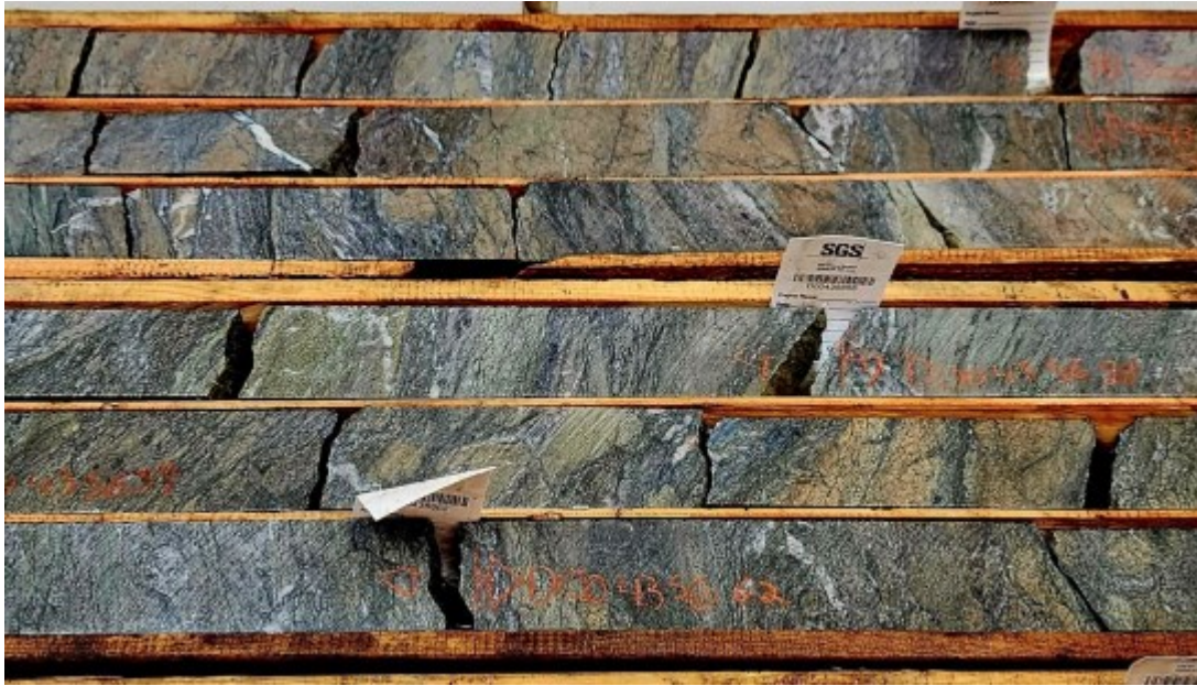
Image 2: Replacement Style Mineralization, DQ23-02 recovery was 90% from 10.65 m of 4.0 g/t Au (Includes 5.0 m of 5.3 g/t Au)
