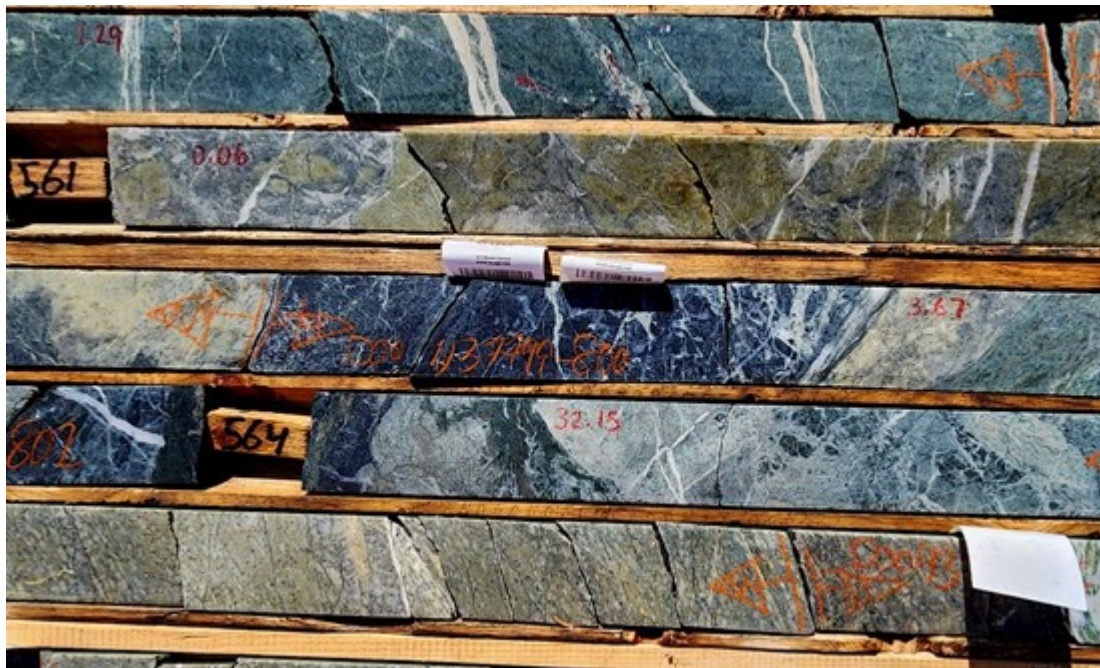
Image 3: Partial Replacement Style Mineralization, DQ23-05 recovery was 94% from 10.8 m of 15.9 g/t Au.
