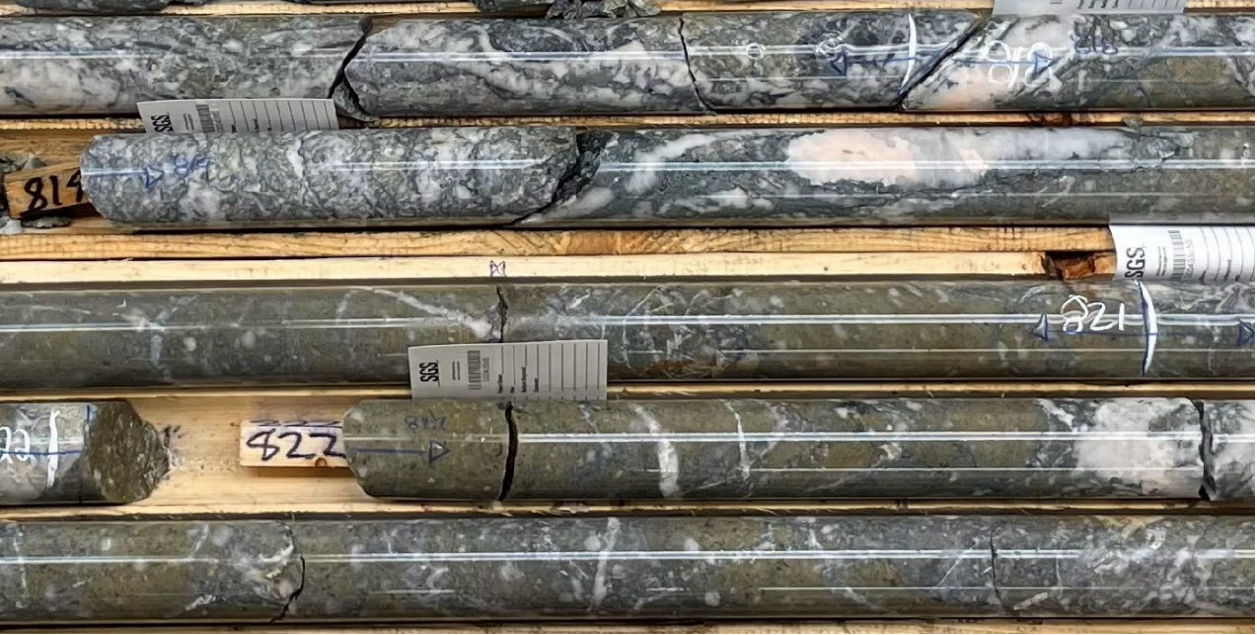
Image 3: Representation of mineralized and altered porphyry core from DQ23-02 (25.0 m of 1.69 g/t Au); bottom of hole ended in mineralization and this zone is subsequently being extended by additional drilling.
