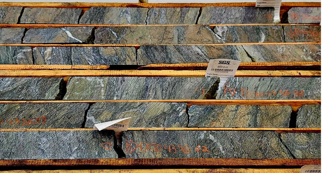
Image 2: Representation of mineralized and altered core from DQ23-02 (10.65 m of 3.97g/t Au (includes 5.0 m of 5.34 g/t Au))
