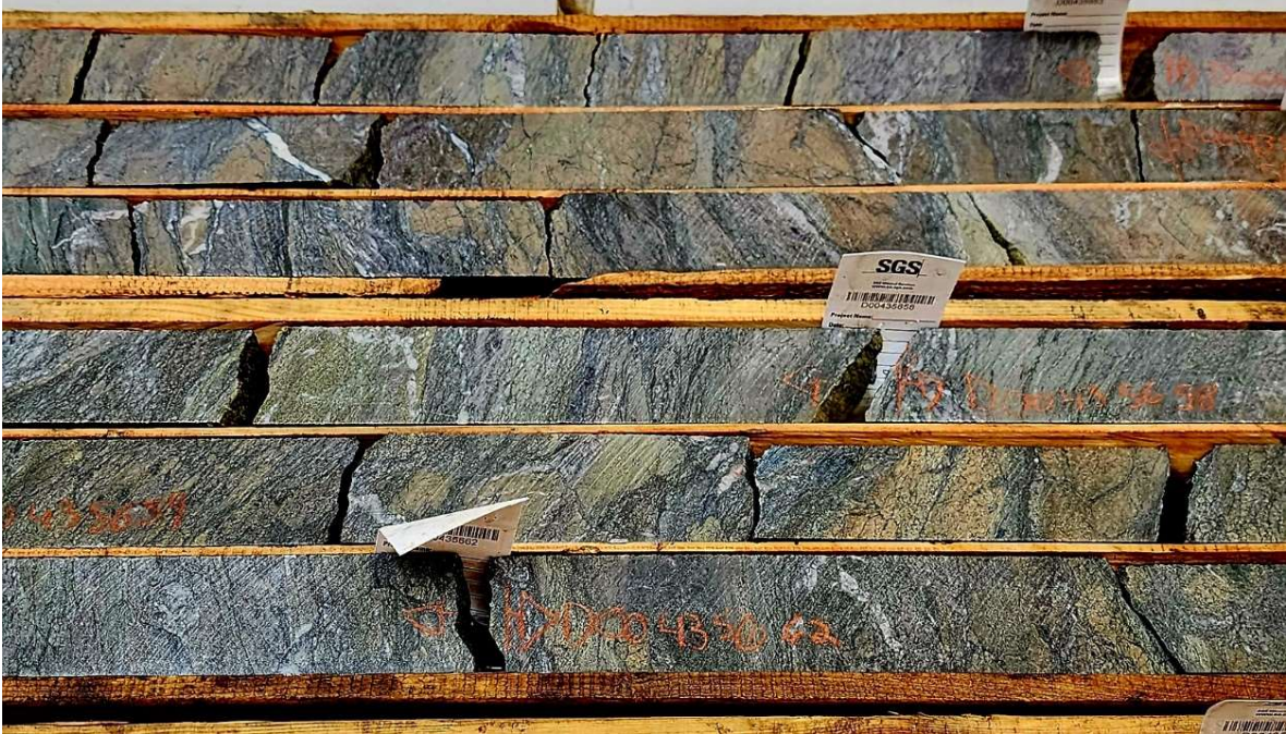
Image 2: Representation of mineralized and altered core from DQ23-02 (10.65 m of 3.97g/t Au (includes 5.0 m of 5.34 g/t Au))
