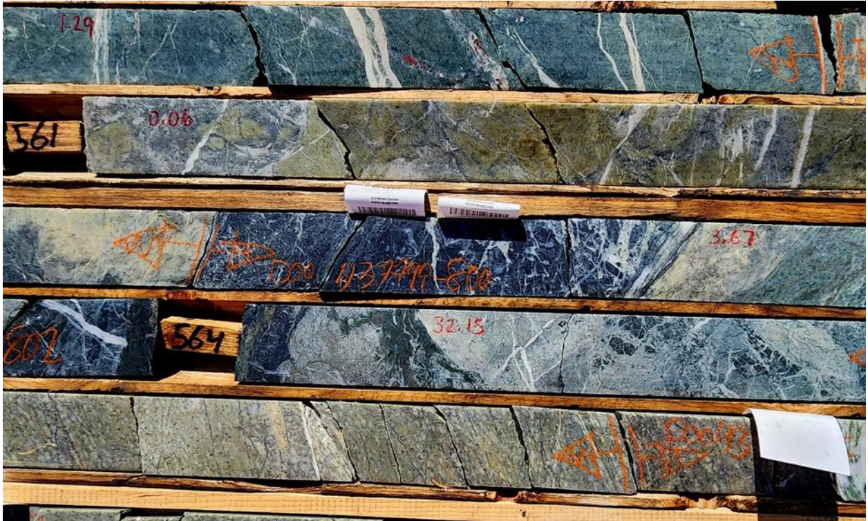
Image 4: Representation of mineralized and altered core from DQ23-05 (10.8 m of 15.8 g/t Au (includes 3.4 m of 27.24 g/t Au)). Highly altered breccia zone containing quartz veinlets, sericite, and ankerite.
