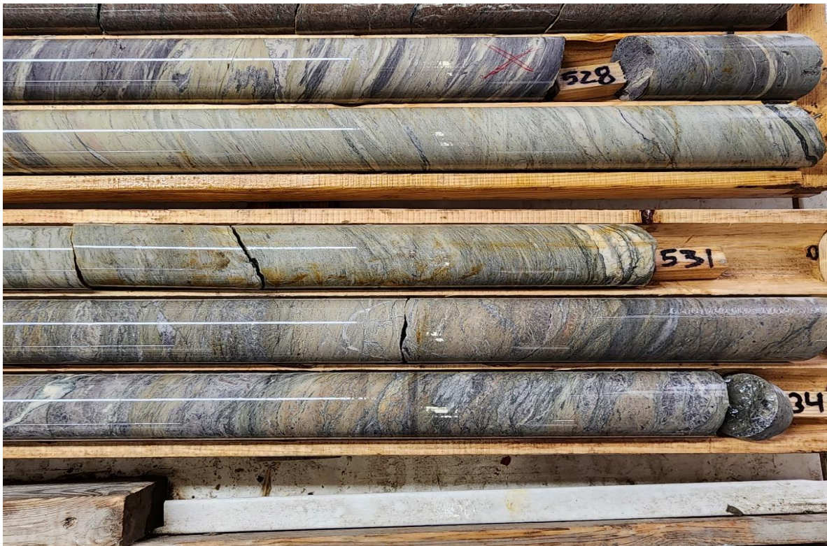
Image 1: Representation of mineralized and altered core from DQ23-01 (11.7 m of 5.63 g/t Au)
