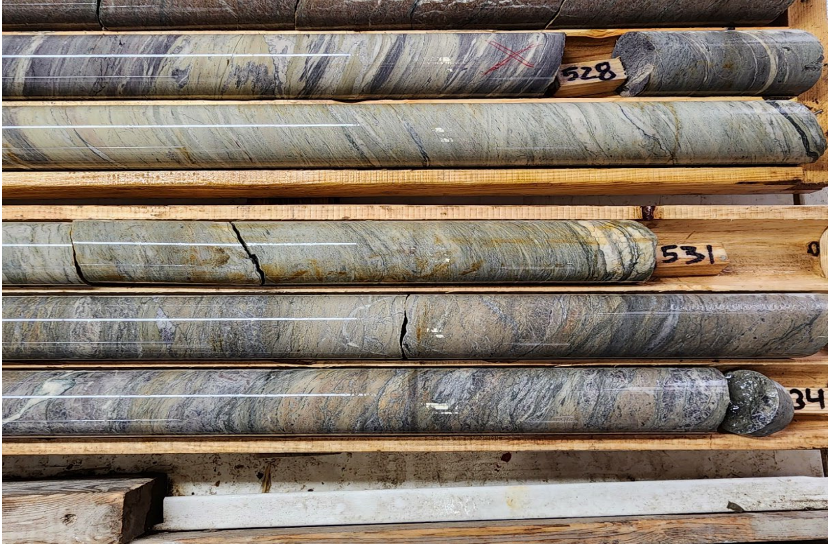
Figure 2: Representation of mineralized and altered core from DQ23-01 (11.7 m of 5.63 g/t Au)
