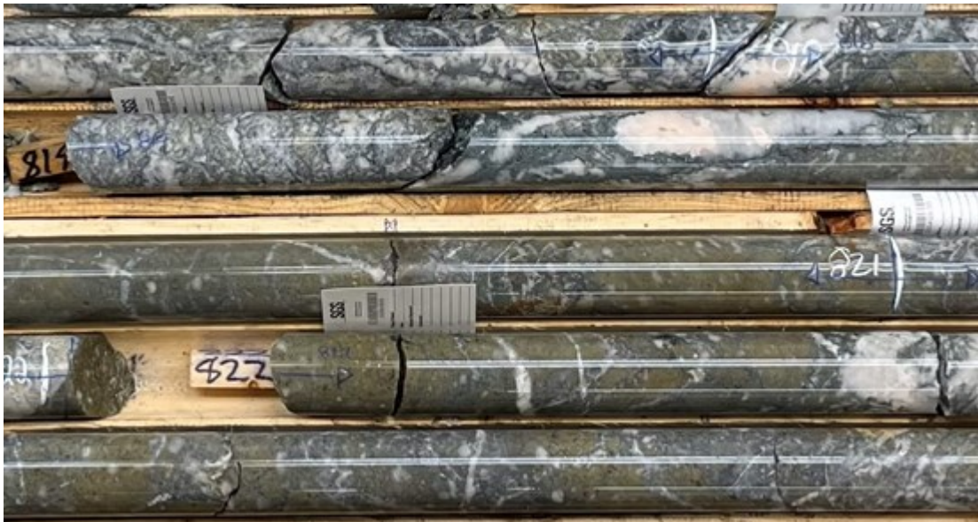
Image 3: Representation of mineralized and altered porphyry core from DQ23-02 (25.0 m of 1.69 g/t Au); bottom of hole ended in mineralization and this zone is subsequently being extended by additional drilling
