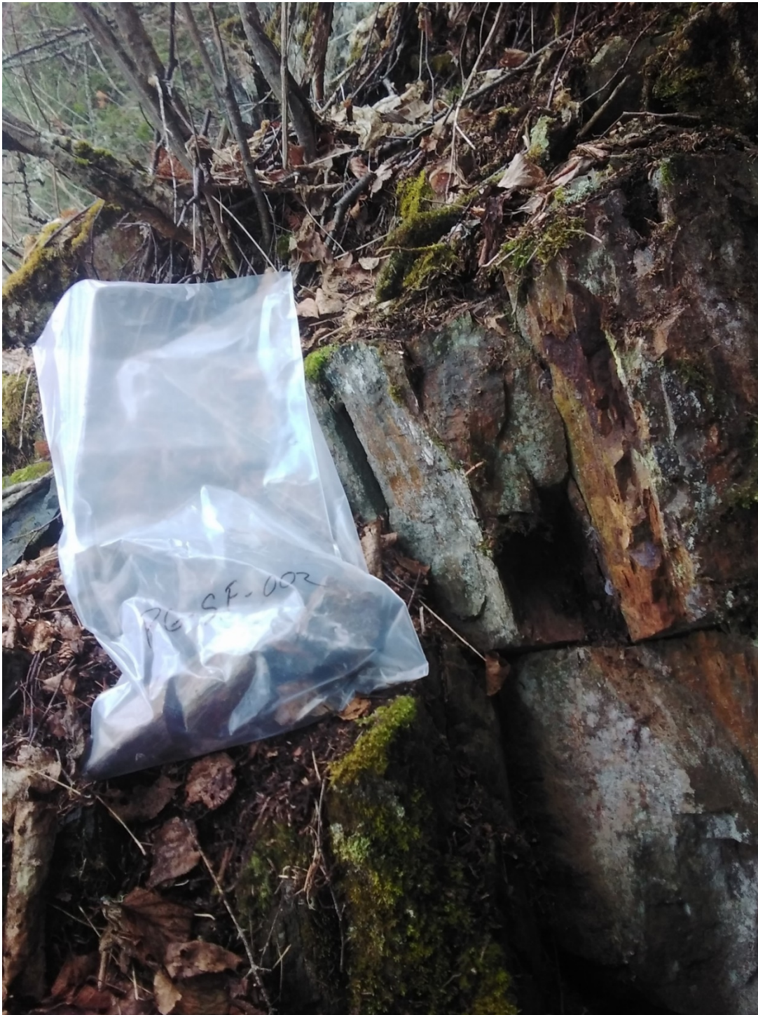
Figure 12.2. Strongly foliated and Fe-stained mafic volcanic tuff near the Turner showing: PG-SF-002.
