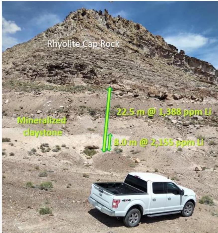
**Figure 2. Rockland Resources Ltd. Lithium Butte Property, Juab County, Utah - Stratigraphic Section showing relative position of channel sample assay results**
