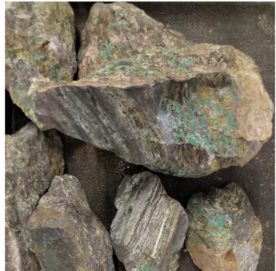
Figure 2 – A060029 – 4Shore disseminated min in meta tuff VG in fractures – 21.3 g/mt Au
