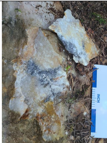
Figure 5. Alcona Mine Zone vein 2 prospect with semi-massive galena (+/- py, po, cpy) mineralization.
