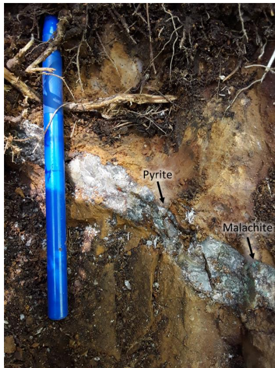
Figure 13. Sample 179308 was collected from the rusty wall rock beside this vein and returned 253 ppb Au, 4.51% Cu and 285 ppm Ni.
