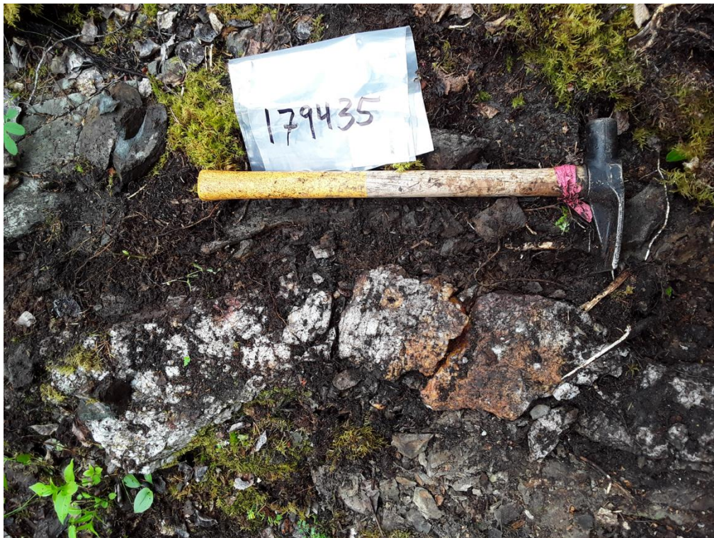
Figure 15. Sample 179435 returned the highest gold result from the 2020 exploration program of 2530 ppb Au. This sample was collected from a 25 - 30cm quartz vein striking 160 / dipping 65.
