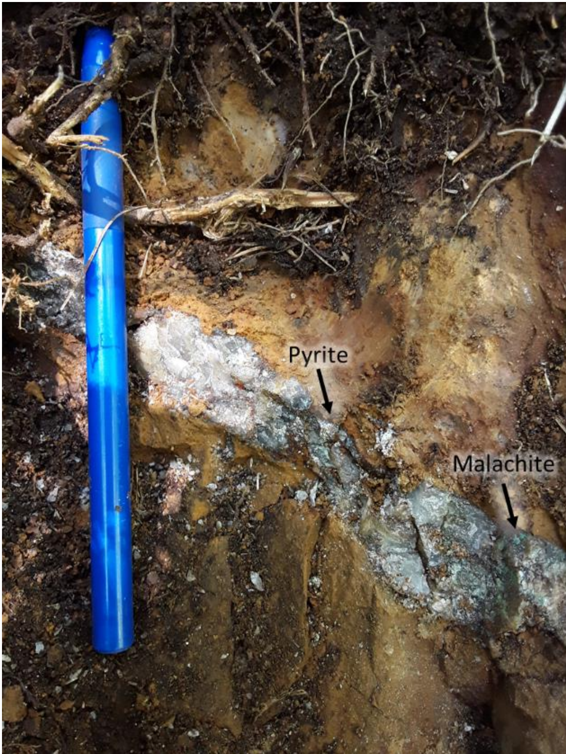
Figure 16. Sample 179308 was collected from the rusty wall rock beside this vein and returned 253 ppb Au, 4.51% Cu and 285 ppm Ni.
