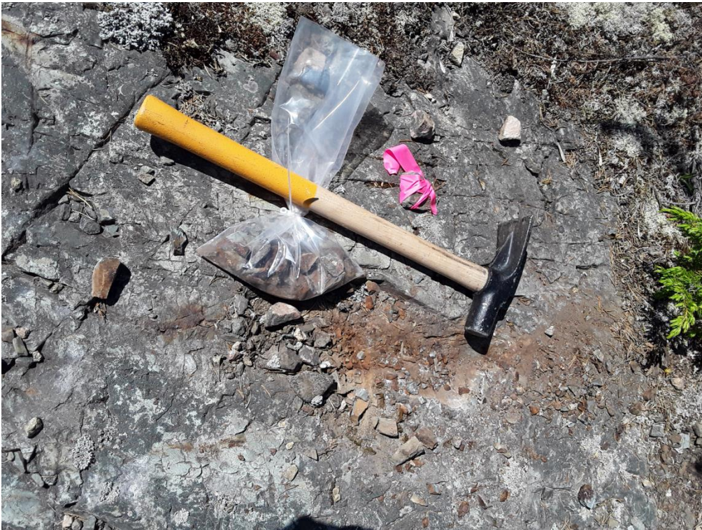
Figure 19. Sample 179266 was collected from a rusty fracture on a smooth siliceous mafic volcanic outcrop and returned 394 ppb Au, 1.36% Cu, and 689 ppm Ni.
