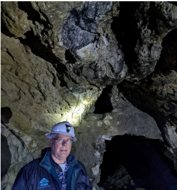
Figure 3. Sample L7 location with Vice President of Exploration Kim Kirkland, inspecting relatively recent artisanal workings. Sample L7 returned 7.7 g/t gold, 916 g/t silver, 0.2 copper, 1.1% lead, and 0.5% zinc.
