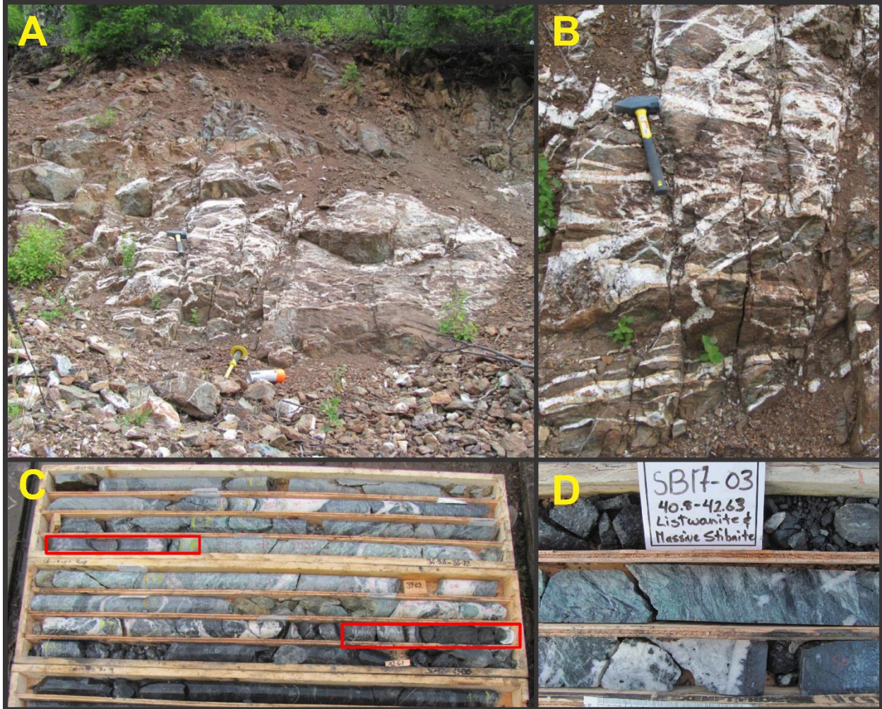
Figure 2. A. Example of Quartz-carbonate vein stockwork near the Peg-leg Vein located southeast of the Main Vein exposed by trenching. (2,5) B. Close up of the same quartz-carbonate vein stockwork. C. Hole SB19-06, high grade intersections from 37.70 to 38.20 returning 18.30 g/t over 0.50m and 41.44 to 42.00 returning 19.25 g/t over 0.56m highlighted in red. D. Hole SB17-03 closeup of quartz-carbonate stockwork veining hosted in listwanite (carbonate altered ultramafic) showing clusters of massive stibnite (antimony) which returned 1.44 g/t over 0.94 meters from 42.56-43.50 meters.
