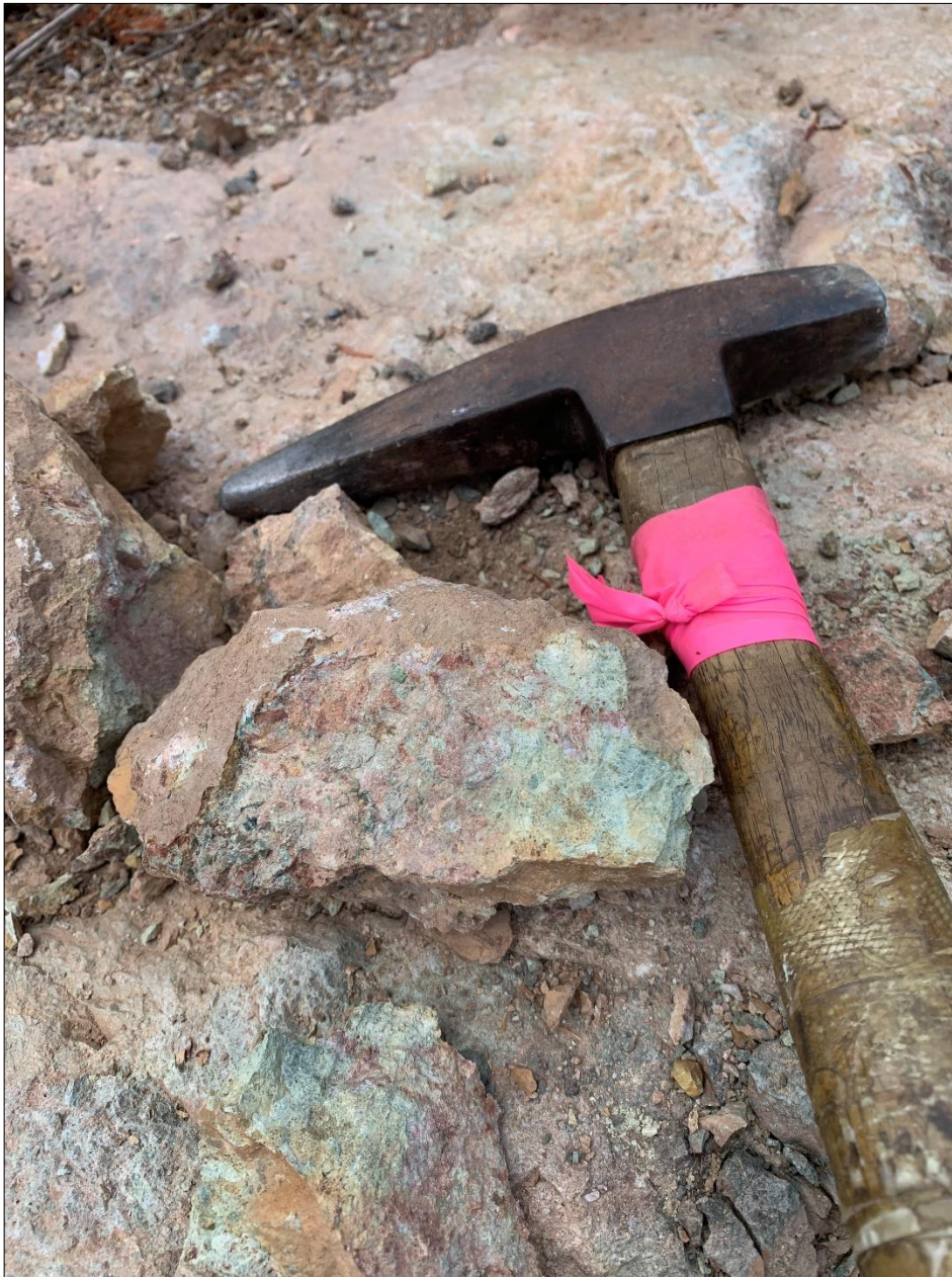
Figure 2-2: Chlorite schist (mafic volcanic) with visible alteration
