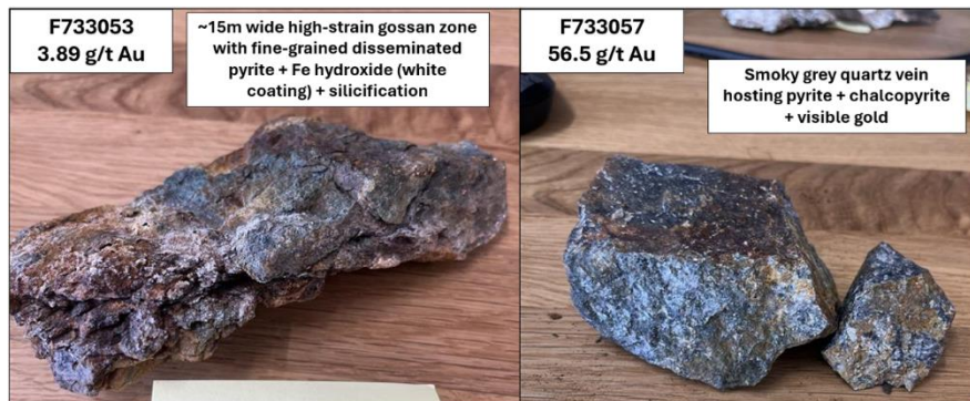
Figure 3: Photographs of grab samples F733053 (left) and F733057 (right) from July 2024 prospecting at Laird Lake.
