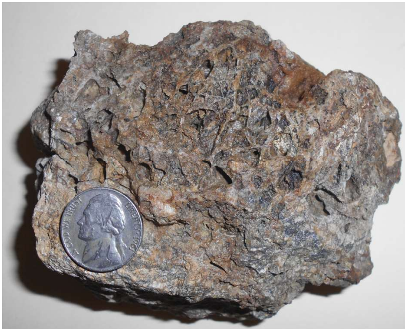
Figure 2. An outcrop of leached quartz stockwork breccia rock recently collected provides compelling evidence of a potentially mineralized porphyry system at depth. This rock sample was collected just north of the proposed south IP line and overlies the magnetic high anomaly.
