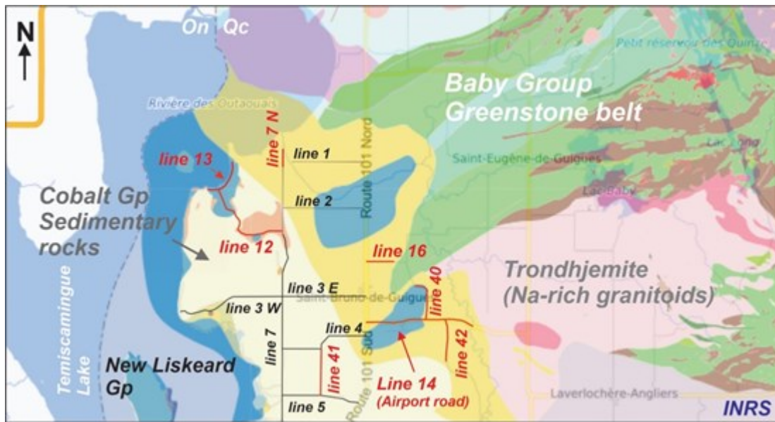
Figure 1: Location plan of the new lines of the September 2024 Soil-Gas survey (in red) and simplified geological map (modified from SIGÉOM, MRNF) highlighting the absence of a green belt (volcanic) in the St-Bruno-de-Guigues airport road sector.
