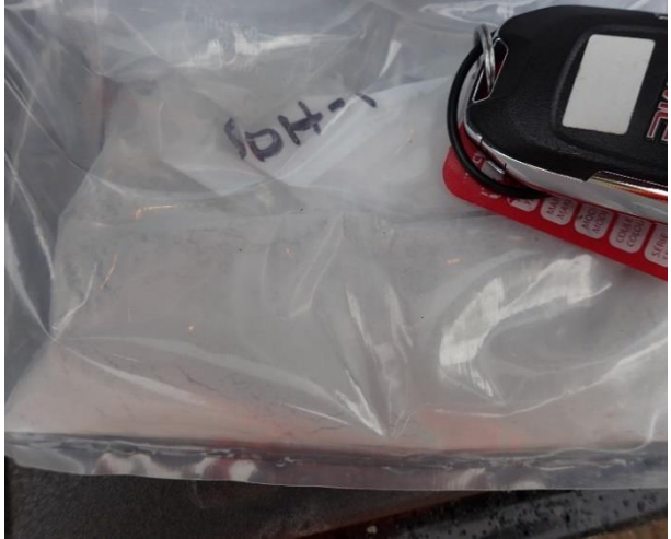
Figure 12-9: Typical drill hole sample (HDH-1), quartzite powder collected by the dust extractor system D25303DH.
