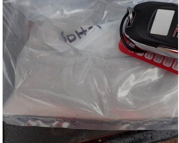
Figure 12-9: Typical drill hole sample (HDH-1), quartzite powder collected by the dust extractor system D25303DH.
