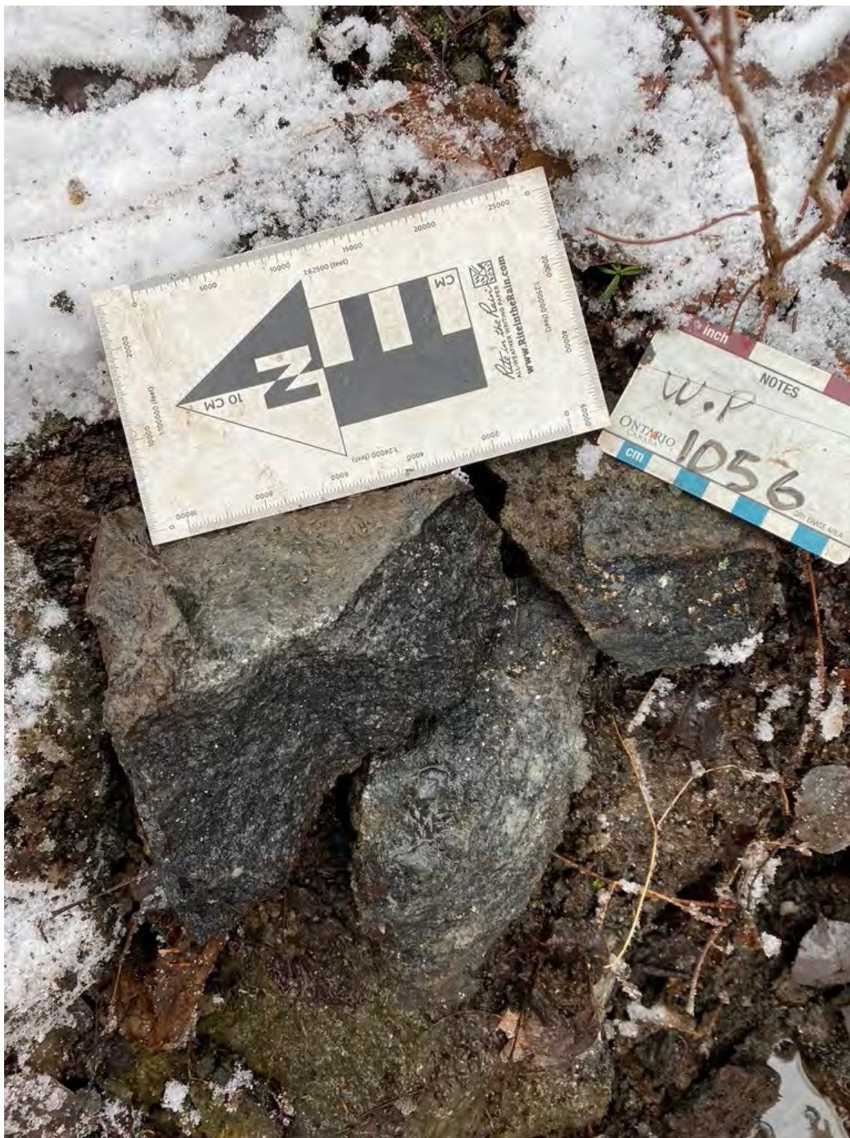
Figure 19: WP 1056: Area J - Sample E5105168 closeup of biotite, quartz, pyrite alteration of mafic volcanic host rocks, found along the Ballard Lake Shear adjacent to quartz veining.
