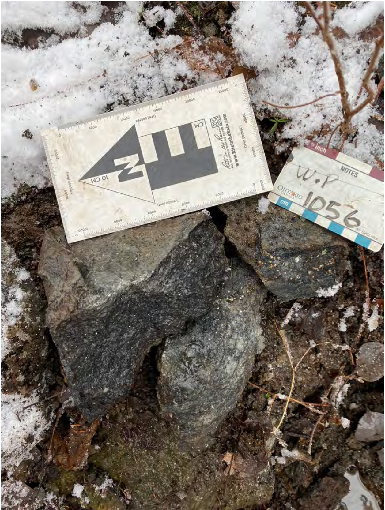
WP 1056: Area J - Sample E5105168 closeup of biotite, quartz, pyrite alteration of mafic volcanic host rocks, found along the Ballard Lake Shear adjacent to quartz veining.
