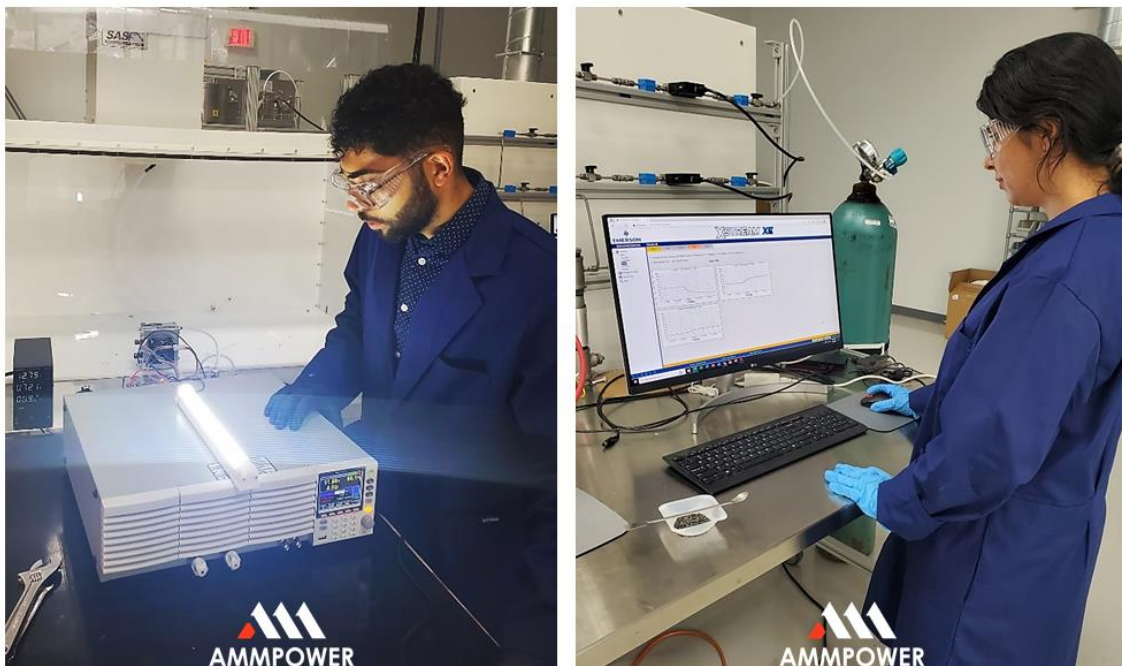
Figure 1. AmmPower’s chemical engineers power an LED light using the electricity from a PEM fuel cell with hydrogen created through the decomposition of ammonia.
