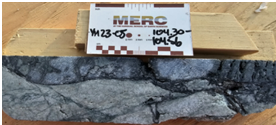
Photo 1: Photographed drill core of YM23-05 from 104.30 – 104.56 meters depth. The core photo illustrates pyrite mineralization within the intrusive unit with pervasive silicification and chlorite alteration.
