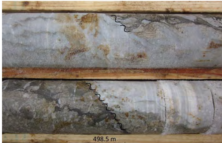
Figure 10-2: Shearing between limestone and anhydrite in DDH 18GHR-005
