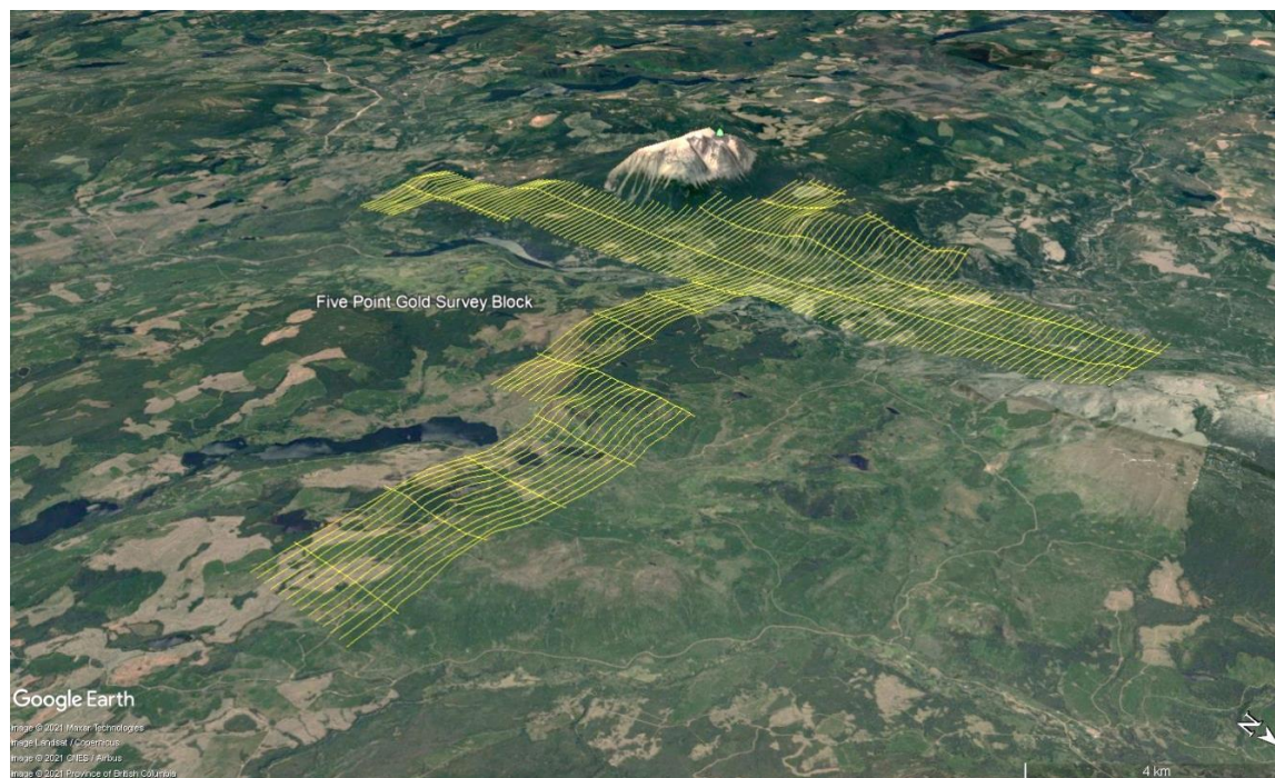
Figure 10: Terrain View –Five Point Gold survey block with actual flight lines in yellow (from Poon and Keyser, 2021).
