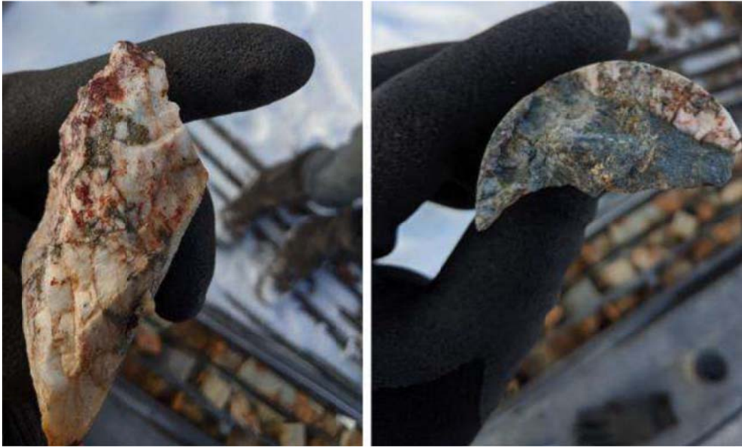
FIGURE 16 – Example of Mineralized Historical Core Found on the Empirical Property
