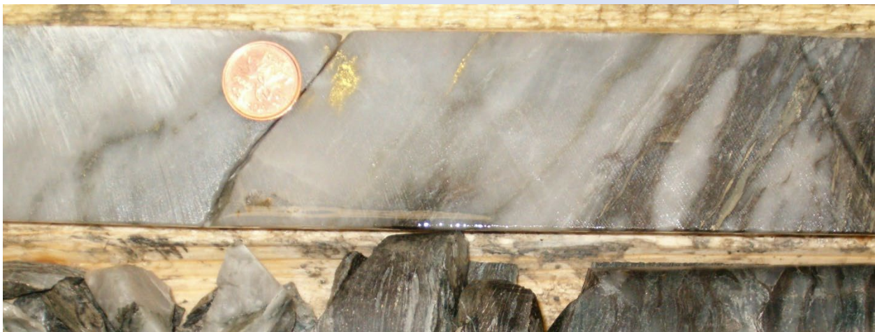
Figure 1 - Photo of Visible gold in drill core from previous operator in a 2006 drill hole. This image is from within an interval of 1.0 m in drill hole DES06-85 from 221.70 m that assayed 167 g/t Au within the DAC zone.
