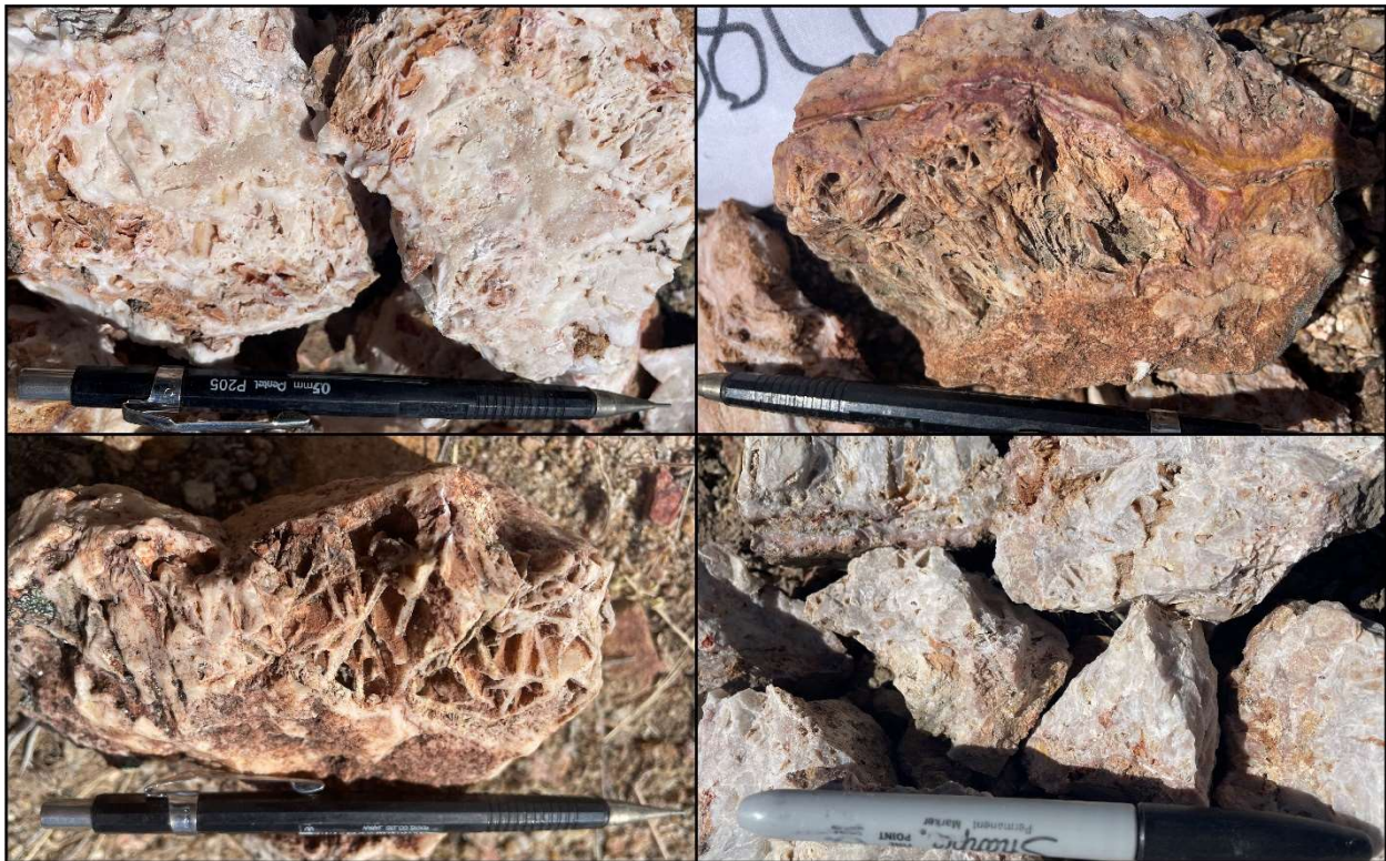
Figure 3: Subcrop and float samples of chalcedonic quartz vein with lattice-bladed calcite and quartz-after-calcite textures, indicative of boiling conditions within an epithermal system.
