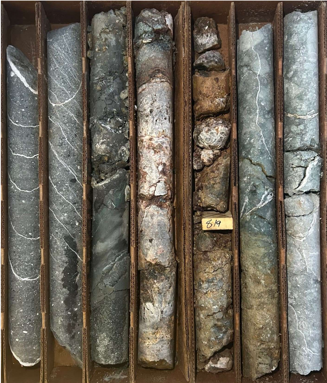
Figure 2: Core photograph of fault-hosted epithermal quartz vein from drill hole MN23-04 exhibiting quartz-after-calcite lattice textures and weak banding of chalcedonic quartz indicative of epithermal boiling. Depth on run block shown in feet.
