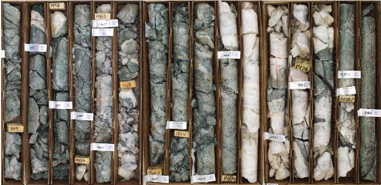
Figure 6. Core photographs of step-out hole SP23-37 from 443.0 m to 451.7 m showing epithermal veining hosted in the Bear Fault zone. True width is estimated at 90% of drilled thickness. Assays pending.
