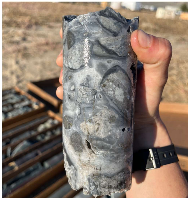
Figure 5. Photograph of epithermal silica-cemented hydrothermal breccia from 379.9 m in drill hole SP23-37. Core is HQ size (6.1 cm diameter). Assays pending.
