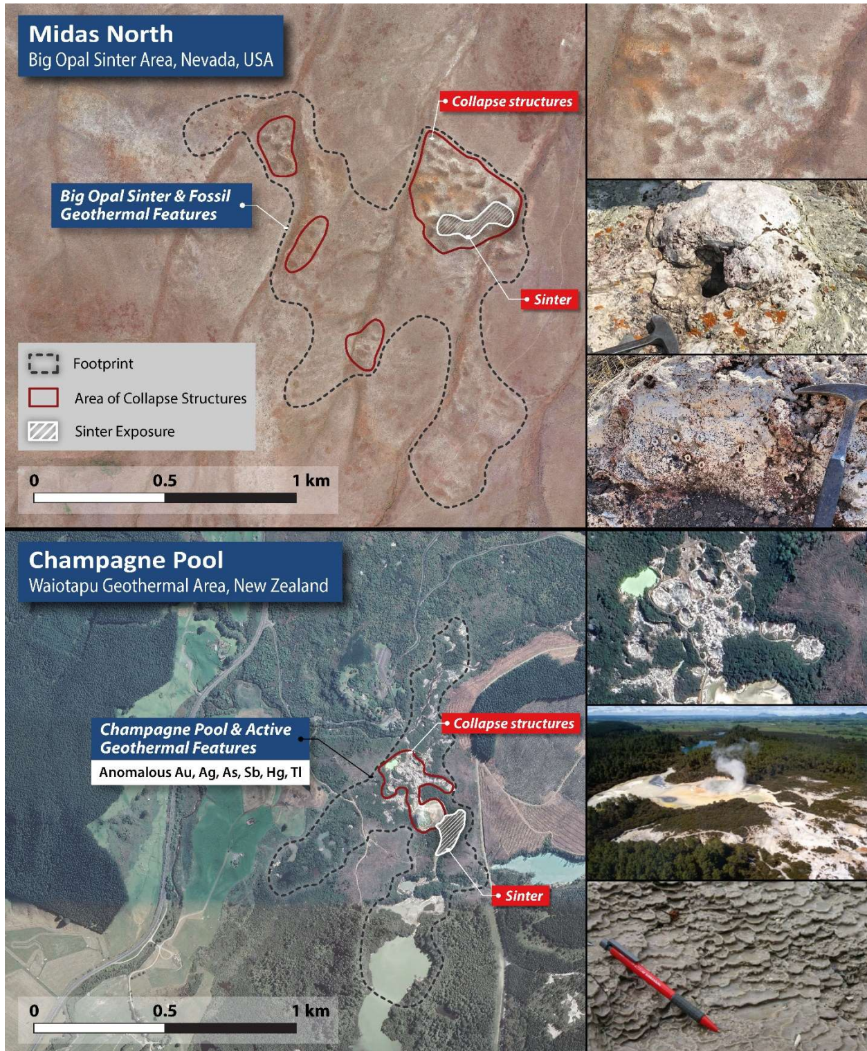
Figure 5: Comparison of sinter and geothermal (hot-spring-related) features at Midas North (top) and Champagne Pool, New Zealand (bottom). Champagne Pool is a globally recognized modern analog for low-sulfidation epithermal systems. Photos demonstrate the comparable sinter characteristics, collapse structures and the relative scale of the two systems, which indicates the potential for Midas North to represent a robust and fully preserved epithermal system.
