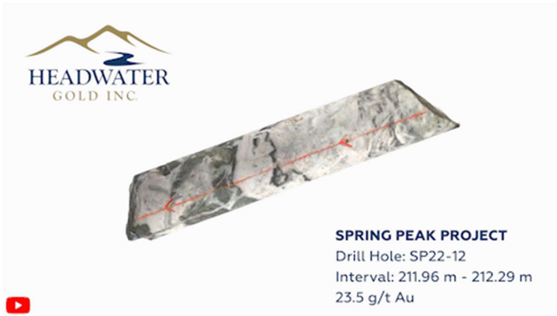
Figure 4: 3D image of ginguero banded quartz vein from the Disco Zone intersected in drill hole SP22-12. Core is HQ size. The pictured vein forms a sample interval which assayed 23.50 g/t Au over 0.33 m from 211.96 m to 212.29 m. Full resolution video is available here
