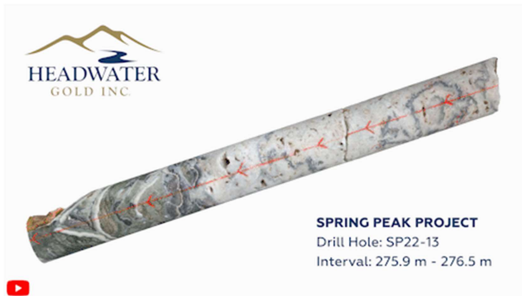
Figure 1: 3D image of ginguero banded quartz vein from the Disco Zone intersected in drill hole SP22-13. Core is HQ size. The pictured vein forms the central portion of the vein interval which assayed 15.92 g/t Au over 2.38 m from 275.26 m to 277.64 m. The right half of the interval shown assayed 69.6 g/t Au over 0.34 m, which is the highest individual assay received from the Spring Peak project to date. Full resolution video is available here .
