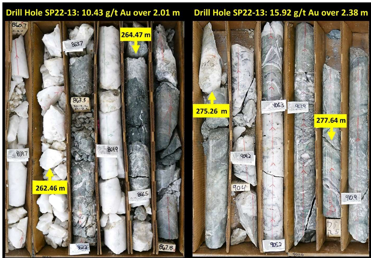
Figure 4: Photos of two high-grade epithermal vein intervals intersected in SP22-13. The upper interval from 262.46 to 264.47 m (left) is dominated by opaque fine-grained silica and abundant bladed quartz after calcite. The lower interval from 275.26 to 277.64 m (right) exhibits abundant gray sulfide-rich ginguro bands, geopedal vein sediments, hydrothermal breccias with rounded vein and wallrock clasts in a silica-sulfide matrix.
