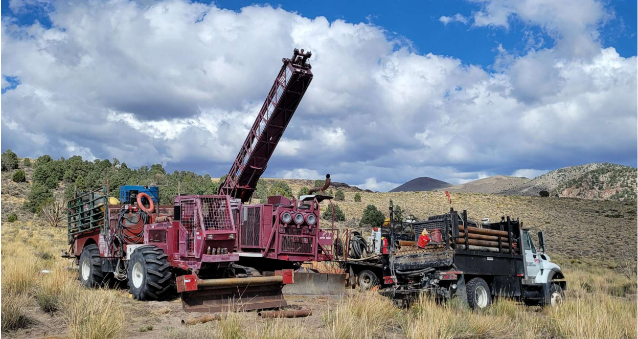
Figure 1: Reverse-circulation drilling currently underway at the Spring Peak Project, Nevada.
