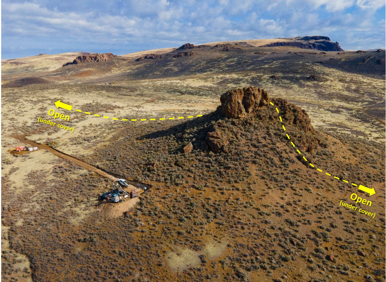
Figure 1: Looking northeast at diamond core rig drilling hole KT21-01 beneath strongly silicified sandstone in the Katey West Zone. The hole was drilled at a -45 degree inclination and encountered high-grade mineralization in a feeder zone directly beneath the resistant outcrop.
