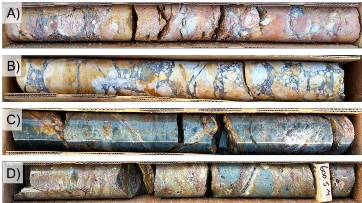
Figure 1: Core photographs of representative epithermal textures encountered in the drilling A) Silicified and hematite-altered breccia in KT21-01; B) Dark gray chalcedonic silica-flooded breccia in rhyolite from KT21-01; C) Strongly silicified rhyolite dike with disseminated sulfides, cross-cut by hematitic fractures in KT21-02; and D) Strongly silicified and oxidized breccia within rhyolite dike swarm in KT21-01. Core is HQ size, and each row is approximately 60 cm in length.
