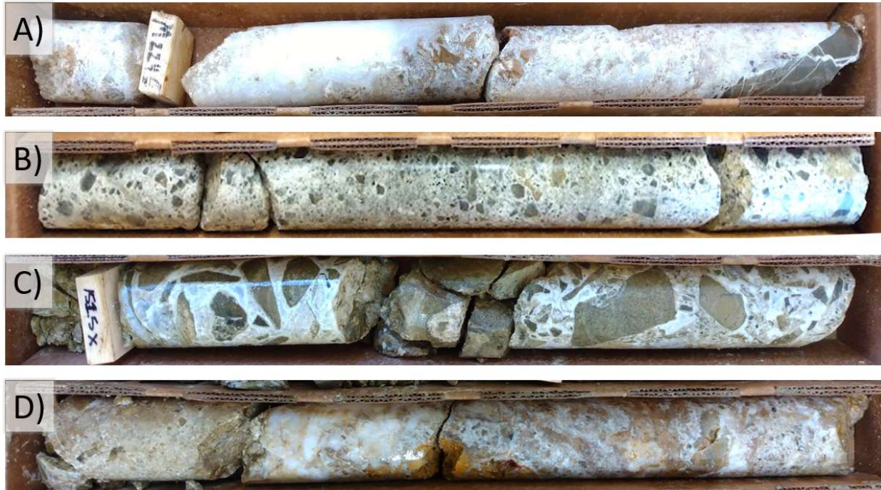
Figure 1: Core photographs of representative epithermal textures encountered in the Headwater 2021 drilling. Core is HQ size, and each row is approximately 60 cm in length. A) Chalcedonic quartz vein from hole MH21-01; B) Heterolithic silica cemented breccia with sub-rounded clasts of milled wallrock from drill hole MH21-01; C) Multiphase vein cemented breccia from drill hole MH21-02; and D) fault-hosted brecciated chalcedonic vein from drill hole MH21-03.
