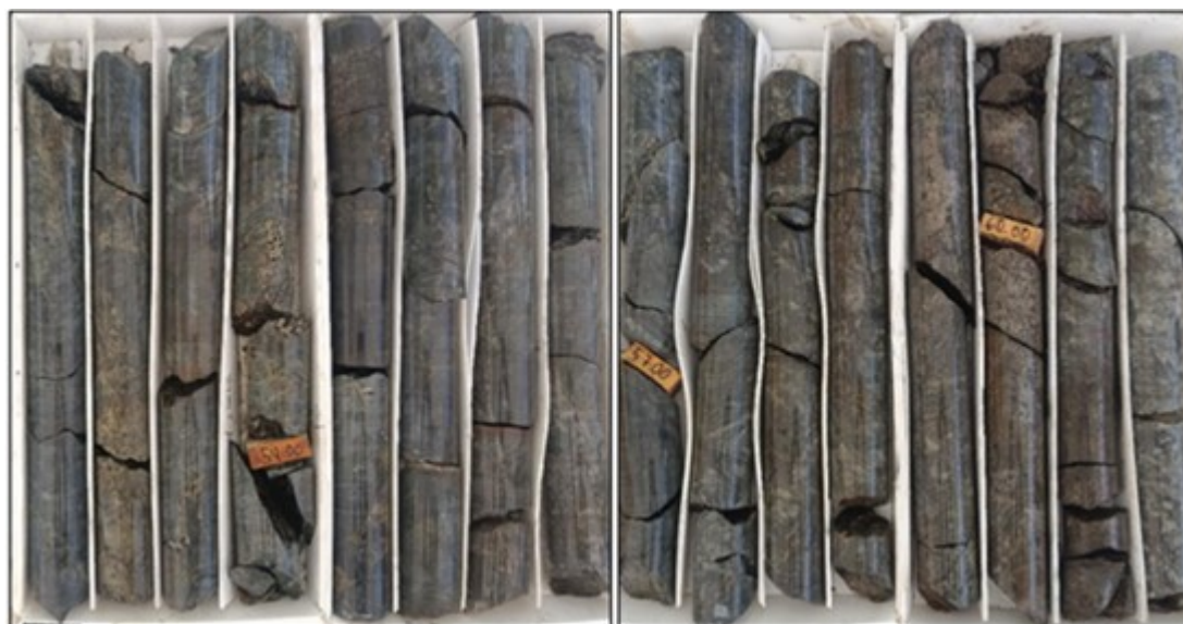
Figure 3. Photographs of sulphide-rich, high-grade core from hole LP-SC-02, including the 6.65 meter core run from 54.88 to 61.53m reported 10.2 g/t Gold and 47.0 g/t Silver .
